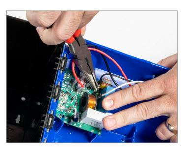
Disconnect any wires connected to the circuit board. There will be two from the transformer and possibly two from the external charging port.
