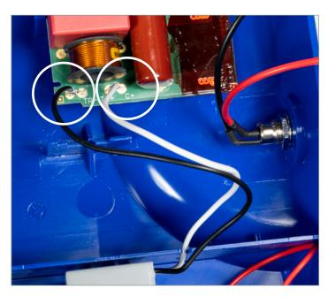
6. Connect black transformer to lead to top left spade terminal. Connect white lead to spade terminal that's just above the capacitor.
