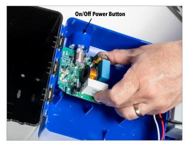
4. Remove old board by lifting the rear and pulling away from power button. Button will pop loose.
