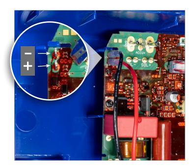
7. IntelliShock units without the external charging port may skip this step. Connect black port lead to "-" spade at top right of board. Connect red port lead to "+" spade just to the left of the "-" spade. Board spades are marked in fine print to indicate polarity.
