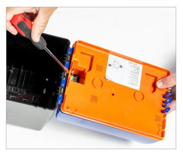
2. Using a standard (flat) screwdriver, insert the tip under the cover where the energizer's lid hinges/connects to the base. Pry off the cover.
