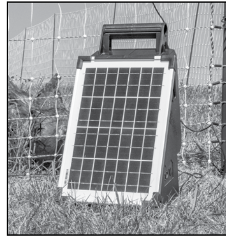
D. Position energizer so that the solar panel faces south in full sun.
