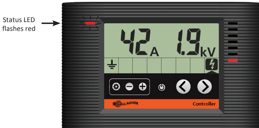
Controller showing the energizer in output alarm
