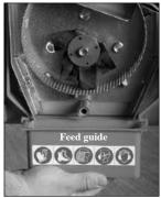
3. Remove mill cover by unthreading knobs. A sieve (e) is already installed. If you wish to change sieve sizes, remove original sieve and replace with new sieve. Sieve fits into mill as shown. Place feed guide (h) into slots below mill.
