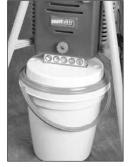
5. Place the lid onto the bucket (b). Press down on the lid (c) and slide the bucket under the feed guide (h).
